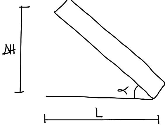
$$\left\{ \begin{array}{l} \tan \alpha = \frac{\Delta H}{L} \\ \Delta H = f \frac{L}{D_n} \frac{v^2}{2g} \end{array} \right.$$
