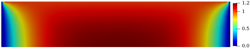
Figure 7: Numerical solution of the heat equation for a triangular mesh with 1357 nodes and 2712 elements. The color represents the temperature with blue being the lowest value and red the highest.
