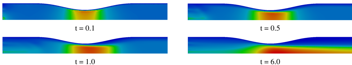
Figure 8: Time evolution of the velocity field for the curved geometry channel. The velocity profile at the middle of the channel is showed in Fig. 7.
