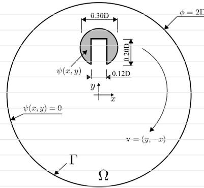
**FIGURE 10** Diagram of the simulation domain for the Zalesak's disk transport. The velocity field is known and imposed by  $\mathbf{v}(x, y) = (y, -x)$ . Therefore, a clockwise rotating flow is achieved. Two full rotations are exhibited during the simulations.
