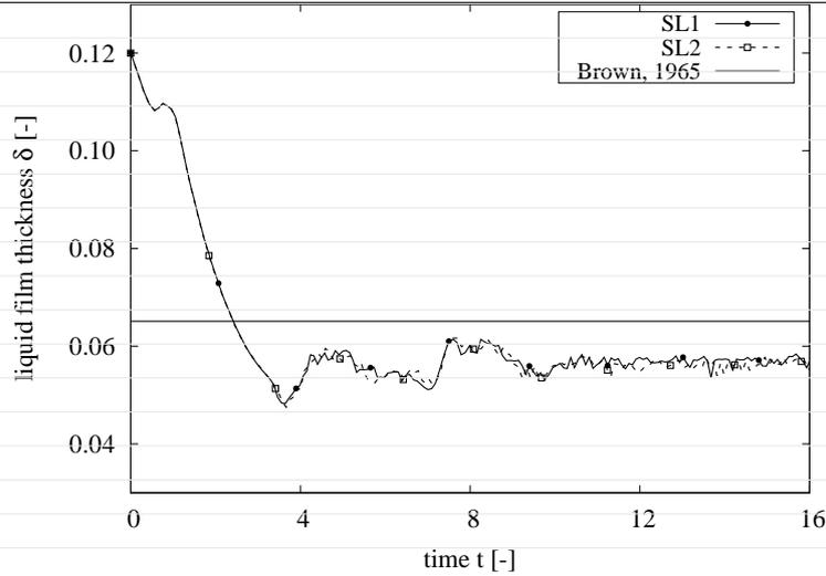
**FIGURE 15** Temporal evolution of the liquid film thickness  $\delta$  for the rising Taylor air bubble immersed in a sucrose solution. This simulation considered  $Mo = 10^{-7}$  and  $Eo = 40$ . The liquid film thickness is computed by using both the SL1 and SL2 schemes and compared afterward with Brown's correlation for elongated bubbles.
