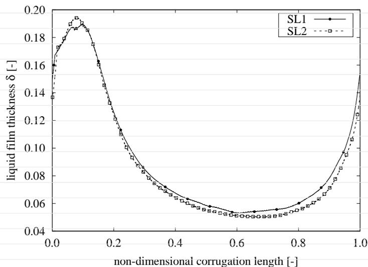
**FIGURE 21** Evolution of liquid film thickness with time for both first- and second-order time Semi-Lagrangian methods for the case of the single bubble ascending through a sinusoidal channel.
