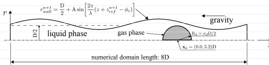
**FIGURE 17** Schematic representation of the domain's geometry and initial air bubble's location for the single drop rising along a sinusoidal capillary channel.
