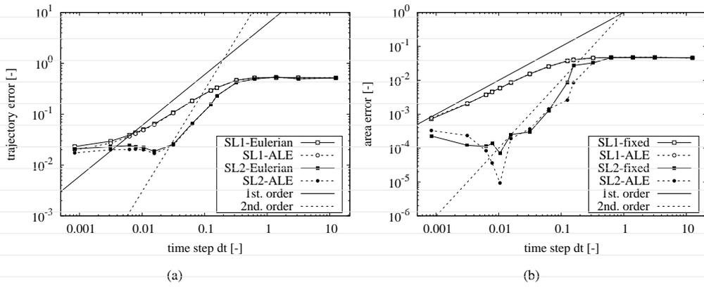
**FIGURE 11** Numerical errors over time computed after 2 revolutions of the Zalesak’s disk test for SL1 and SL2 schemes: (a) trajectory error; (b) area error. As can be seen, in the SL1 scheme the convergence error is found to be linear for the area error and sub-linear for the trajectory error. On the other hand, the SL2 scheme presented second order of convergence in the area error and sub-quadratic order of convergence for the trajectory error.
