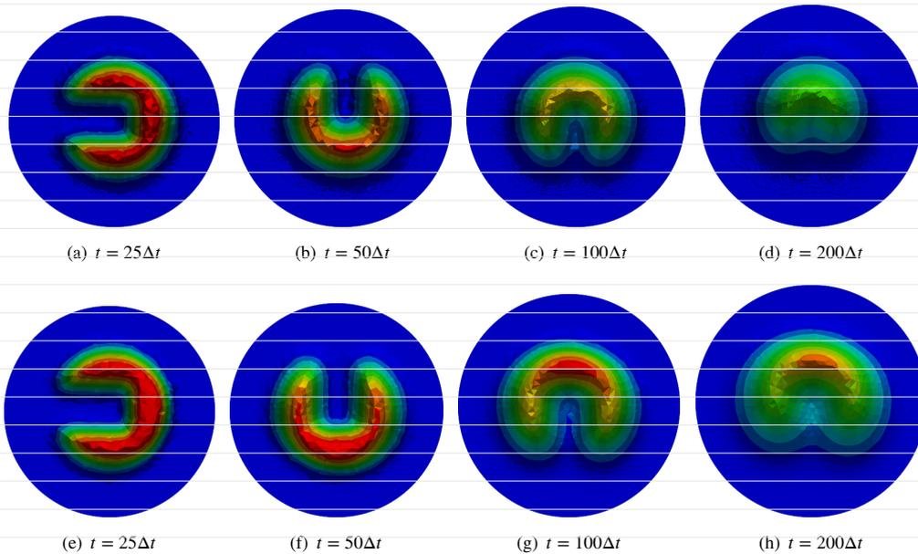
**FIGURE 12** Comparison snapshots of Zalesak’s disk profiles during revolutions impelled by the rotation flow for several simulation times within 200 iterations. First row: scalar blob approximated by the SL1 scheme. Second row: scalar blob approximated by the SL2 scheme.
