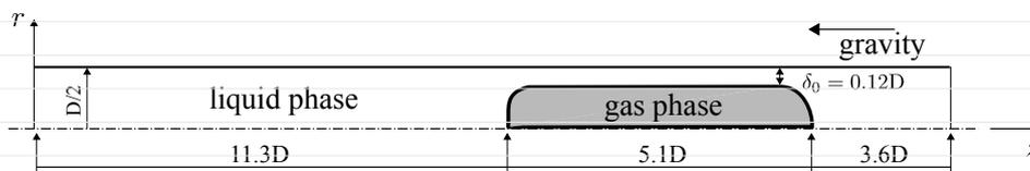
**FIGURE 13** Schematic representation of the domain's geometry and initial air bubble's location for the two-phase flow of a rising Taylor air bubble.
