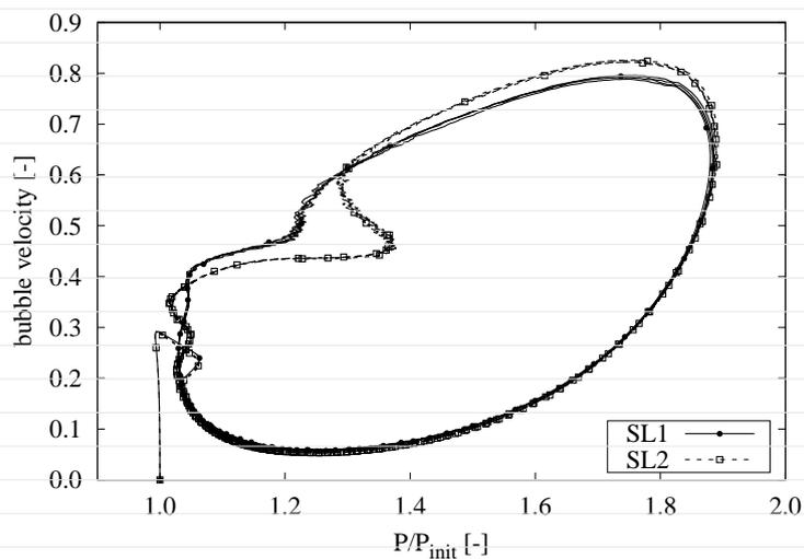
**FIGURE 19** Phase diagram relating the bubble's perimeter ratio  $P/P_{init}$  and the bubble's center of mass. Stable orbits show well-defined limit cycles for both SL1 and SL2 methods and absence of chaos, thus verifying that the numerical code reproduces the physical behavior with high fidelity.
