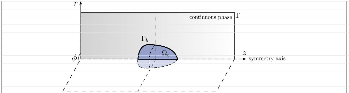
**FIGURE 1** Generic model for an axisymmetric continuous-dispersed two-phase flow. Dispersed bodies are represented by the inner region  $\Omega_b$  with boundary  $\Gamma_b$  that moves along the symmetry axis  $z$  and undergoes interface changes along the radial coordinate  $r$ .
