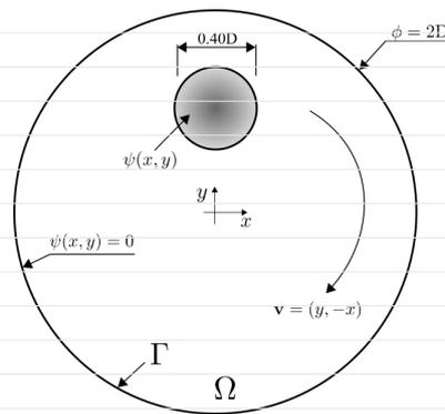
**FIGURE 8** Diagram of the simulation domain for the Gaussian function transport. The velocity field is known and imposed by  $\mathbf{v}(x, y) = (y, -x)$ . Therefore, a clockwise rotating flow is achieved. Two full rotations are exhibited during the simulations.
