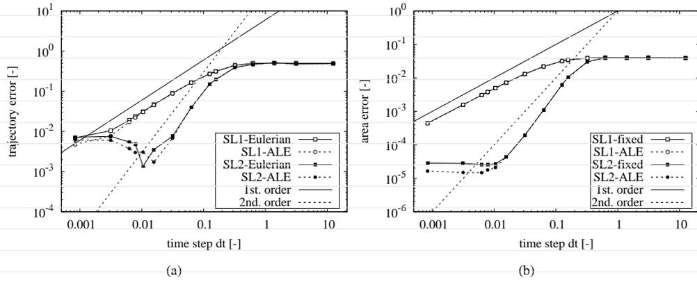
**FIGURE 9** Numerical errors over time computed after 2 revolutions of the Gaussian profile test for SL1 and SL2 schemes: (a) trajectory error; (b) area error.
