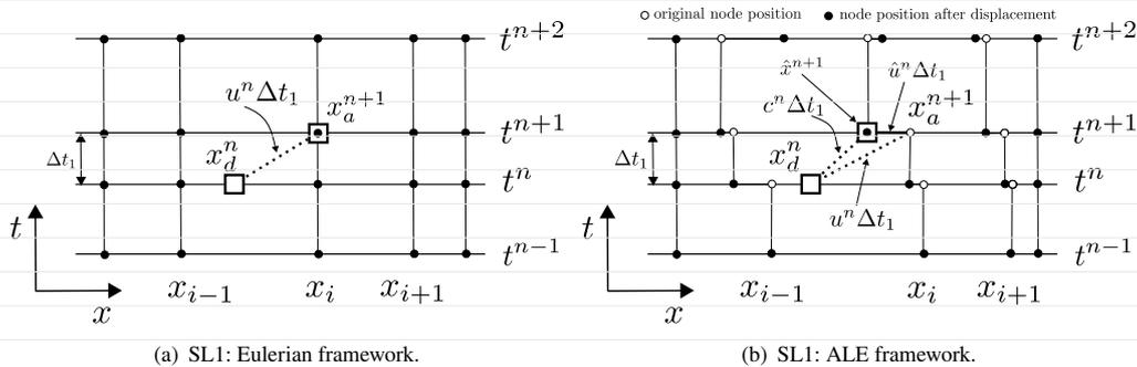
**FIGURE 4** One-dimensional space-time stencils representing the first-order SL scheme. The point  $x_d$  is found by integrating the fluid trajectories backward-in-time. Afterward, the flow variables are interpolated by considering the degrees of freedom placed at the nodes  $x_{i-1}$  and  $x_i$ .
