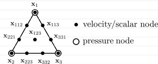
**FIGURE 2** Stable element used in this paper: the “10-node triangle”,  $(P_3, P_1)$ , or cubic element.
