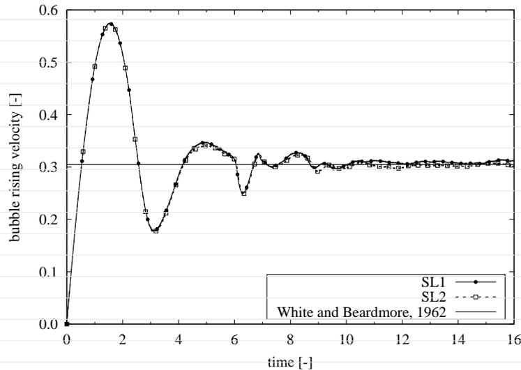
**FIGURE 14** Rising velocity profile of a single Taylor air bubble immersed in a sucrose solution for  $Mo = 10^{-7}$  and  $Eo = 30$ . Both profiles show that the bubble's center of mass velocity obtained with schemes SL1 and SL2 are in narrow agreement with experiments.
