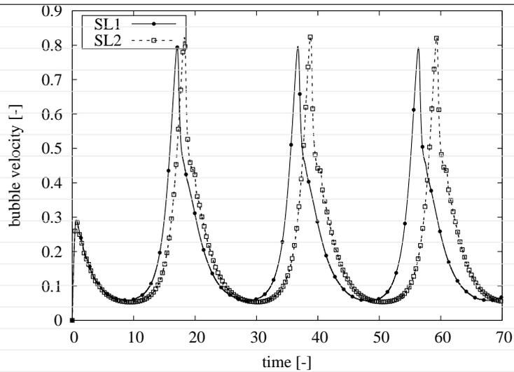
**FIGURE 20** Temporal evolution of the velocity at the bubble's center of mass comparing the SL1 and SL2 methods along three corrugated lengths.
