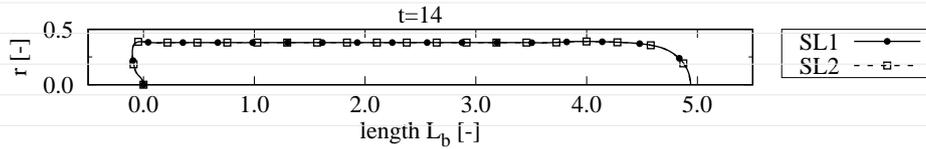
**FIGURE 16** Comparison of the air bubble's terminal shape for both time integration schemes moving in a sucrose solution. This simulation considered  $Mo = 10^{-7}$  and  $Eo = 30$  and the snapshot was taken in dimensionless time  $t = 14$ .
